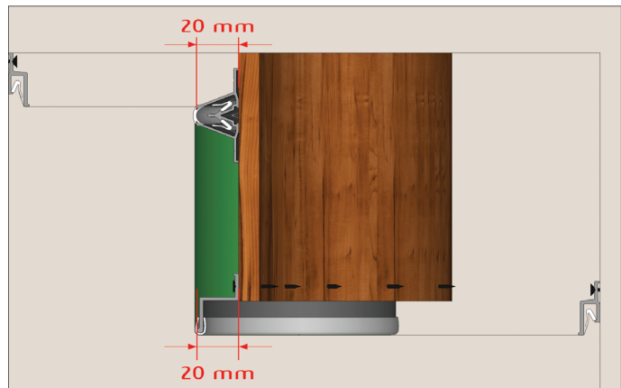
Fastening the profile to the concrete ceiling
