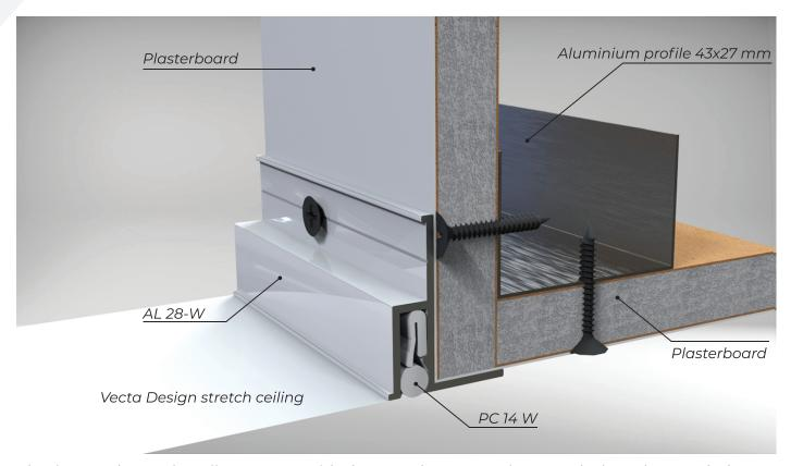
Elastic PVC decoration clip PC-14 W with the round cross-section was designed to mask the gap in the lock, it is very easy and convenient to use. The profile has a lock for using the MINIharpoon. AL 28-W is colored in neutral white semi-mat RAL 9003.
