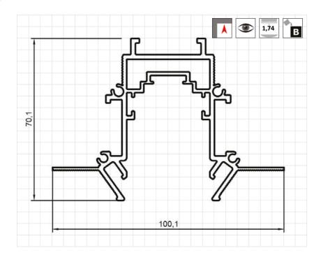
There are four screw grooves on the side of the profile structure, which make it easy to attach the end cover and create profile structures of different lengths according to customers wishes. The profile structure lower part includes recesses for fastening the stretch material harpoons and edges on both outer sides for fastening alternative ceiling materials.
